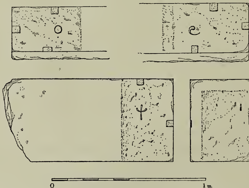
FIG. 13. FRAGMENTS OF INNER EPISTYLE BEAMS, SHOWING SHIFT-HOLES AND MASONS' MARKS.
